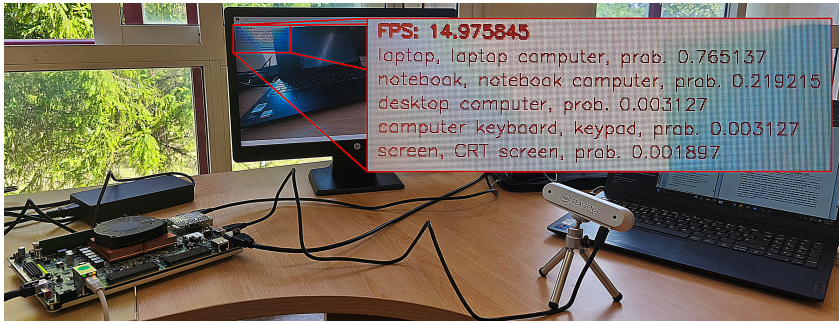
Figure 5: Real-time classification using the color (RGB) sensor of the Intel RealSense D455 camera. The camera limits performance to 15 FPS.
