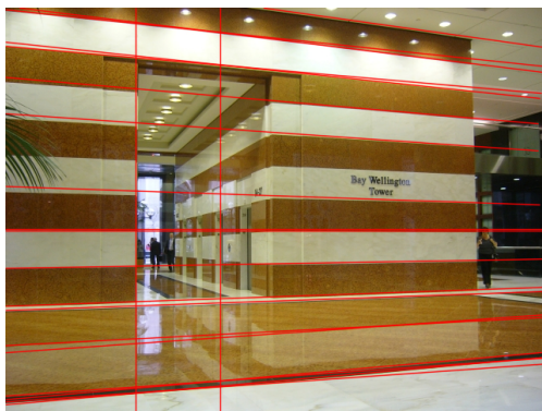
Figure 2: Example of a Hough lines detection result on an image from the York Urban Line Segment Database [Denis et al. (2008)]. Detected lines are overlaid over the original image
