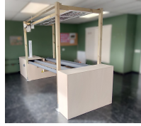
Figure 1: Physical structure showing the wooden frame, PVC cultivation pipes and protective panels.
