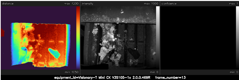
Figure 2: Example of raw data (from left to right): distance (pseudocolor), intensity and confidence.
