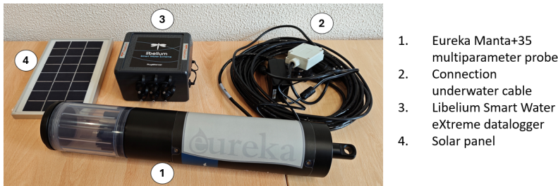
Figure 3: Monitoring equipment used in the study: Eureka Manta+35 multiparametric probe, Libelium Smart Water eXtreme datalogger with solar panel, and connection cable ( Source: own elaboration )
